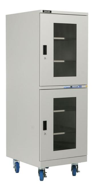
CSD-702-03 has an outstanding performance for drying moisture sensitive components and PCBs as a result of a high performance drying unit. Humidity can be controlled precisely by digital panel to reach the lowest <3%RH. It is specially designed for moisture sensitive SMD packages to comply with IPC/JEDEC J-STD-033D.
