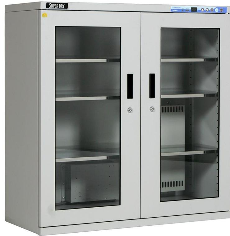
SD-252-02 has an outstanding performance for drying moisture sensitive components and PCBs as a result of a high performance drying unit. Humidity can be controlled precisely by digital panel to reach the lowest 2%RH. It is specially designed for moisture sensitive SMD packages to comply with IPC/JEDEC J-STD-033D.
